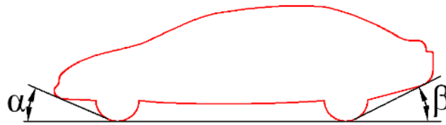
Fig 9: Car shape with front and rear maneuverability angles
